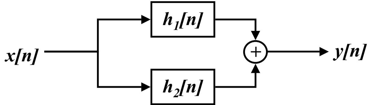
$$y[n] = (x[n] * h_1[n]) + (x[n] * h_2[n]) = x[n] * (h_1[n] + h_2[n])$$
