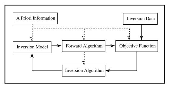
Figure 1: Elements of an Inverse Modeling Procedure.
